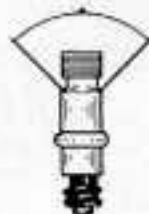
Fig. 7. This Ruhmer cell is mounted in an evacuated tube which is silvered on the sides to reflect light on the cell
