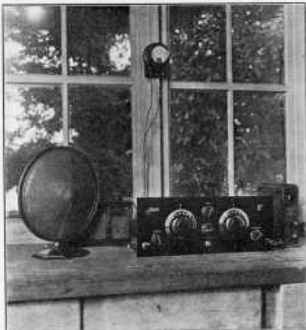
Fig. 1. The T. C. set at the Darien laboratory, operating from a Timmons B-Liminator. Note the double-range Jewell voltmeter, used to get the correct rheostat settings
