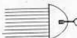
Fig. 4. The Bell-Tainter cell mounted in a parabolic reflector.
